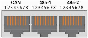
If you need to communicate with the monitoring device through RS485 or Can, the monitoring device will be used as the host, and the address setting range of other batteries will be 2~15 according to the polling data of the address.
